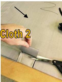
**Step 11:** Introduce the counterweight plate completely, and we proceed to cut the excess textile from the cloth 2.
