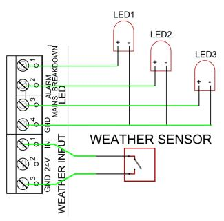
LED - signaling diode outputs: breakdown (failure, LED1), ALARM (LED2), MAINS (power supply, LED3).
