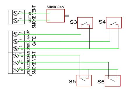
SMOKE VENT MOTOR - 24VDC smoke damper motor.
