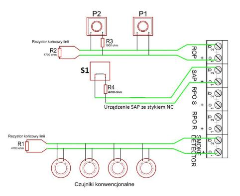
ROP - manual call point input, i.e. the alarm button. Several such buttons can be connected in parallel. There are two types of buttons, one with a built-in 1000 Ohm resistor (P1 in the figure), the other without (P2 in the figure), in the absence of a built-in resistor, such resistor (R3 in the figure) should be connected in series with the button as shown. At the end of the line, connect a 4700ohm resistor (R2).
