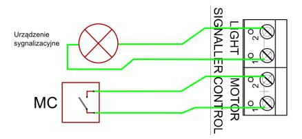
24VDC signaling device output, e.g. bulb or other, which turns on during an alarm.
