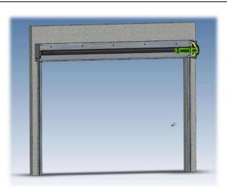
Mount the motor to the holder and connect the drive chain. Turn the screws on the motor to adjust the chain tension. The motor is equipped with a safety device for releasing the brake and controlled closing in case of emergency.
