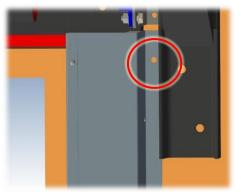
Fasten the guide casing to the masonry (using suitable fasteners for the masonry) through the series of holes on the external
