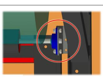
Secure the drive shaft to the bracket using the supplied flange bearings. The distance must be adjusted according to the fabric.
