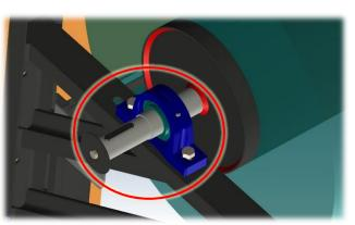
Bearing fixing on engine bracket
