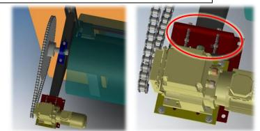
Bolt the motor to the respective adapter plate, slide it into the appropriate tracks on the bracket Insert the pinions their respective axes. in Position the chain and align the sprockets and then act on the respective dowels to lock them. At the end, it is necessary to replace the stop washer on the axis.
