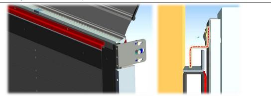
Once the previous operations have been carried out, check the correct fastening position which, when the sheet is completely unrolled, must be just above the "cross" profile fixed to the lintel. Once this position has been marked on the element, the sheet must be wound so that it is easy to access, drill 5mm holes (not through holes) and fix the Z profile with 4.8x8mm steel rivets, in correspondence with the rivets on the element insert a 4.8x19mm self-drilling screw.
