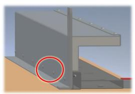
Fix the cover to the guide plates by inserting self-drilling screws (supplied) in the series of holes on the internal and external side.
