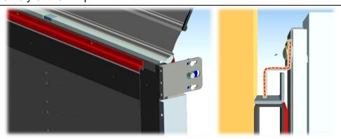
Once the previous operations have been carried out, check the correct fastening position which, when the sheet is completely unrolled, must be just above the "cross" profile fixed to the lintel. Once this position has been marked on the element, the sheet must be wound so that it is easy to access, drill 5mm holes (not through holes) and fix the Z profile with 4.8x8mm steel rivets, in correspondence with the rivets on the element insert a 4.8x19mm self-drilling screw.
