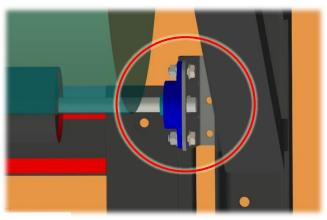
Secure the motor shaft to the shelf using the supplied flange bearings. The distance must be adjusted according to the mantle.
