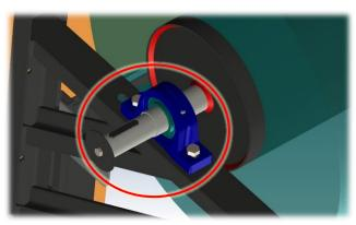
Bearing fixing on motor shelf
