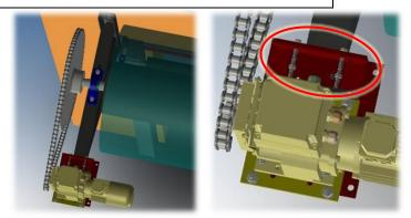
Adjust the chain by acting on the chain tensioner screws.
