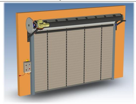
Cut the containment straps and through the control unit slowly unroll the mantle inside the guides. Adjust the little shaft so that it accompanies the mantle keeping it vertical.
