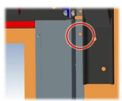
Fasten the guide covers to the masonry (using suitable fasteners for the masonry) through the series of holes on the external fin.
