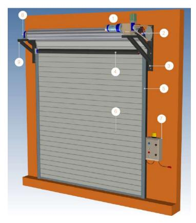
A robust "U" shaped profile with a thermos-expanding gasket applied completes the bottom element. The slats are infilled with three layers of highly performing silicate material that guarantee, after one /two hours of fire exposition in according to the fire test procedure reported on EN 1634-1, a detected average temperature lower than 140°C on the other side not exposed to fire.
