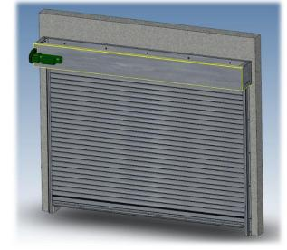
Insert the Front Box behind the motor leaning it against the side brackets. Fix it with the special screws supplied to the lower threaded holes of the flags.
