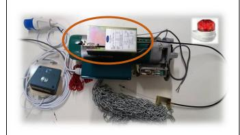
**ATTENTION:** If the Solenoid is not armed, the actuator pushes on the motor brake release lever keeping it open. The motor does not lift the shutter.
